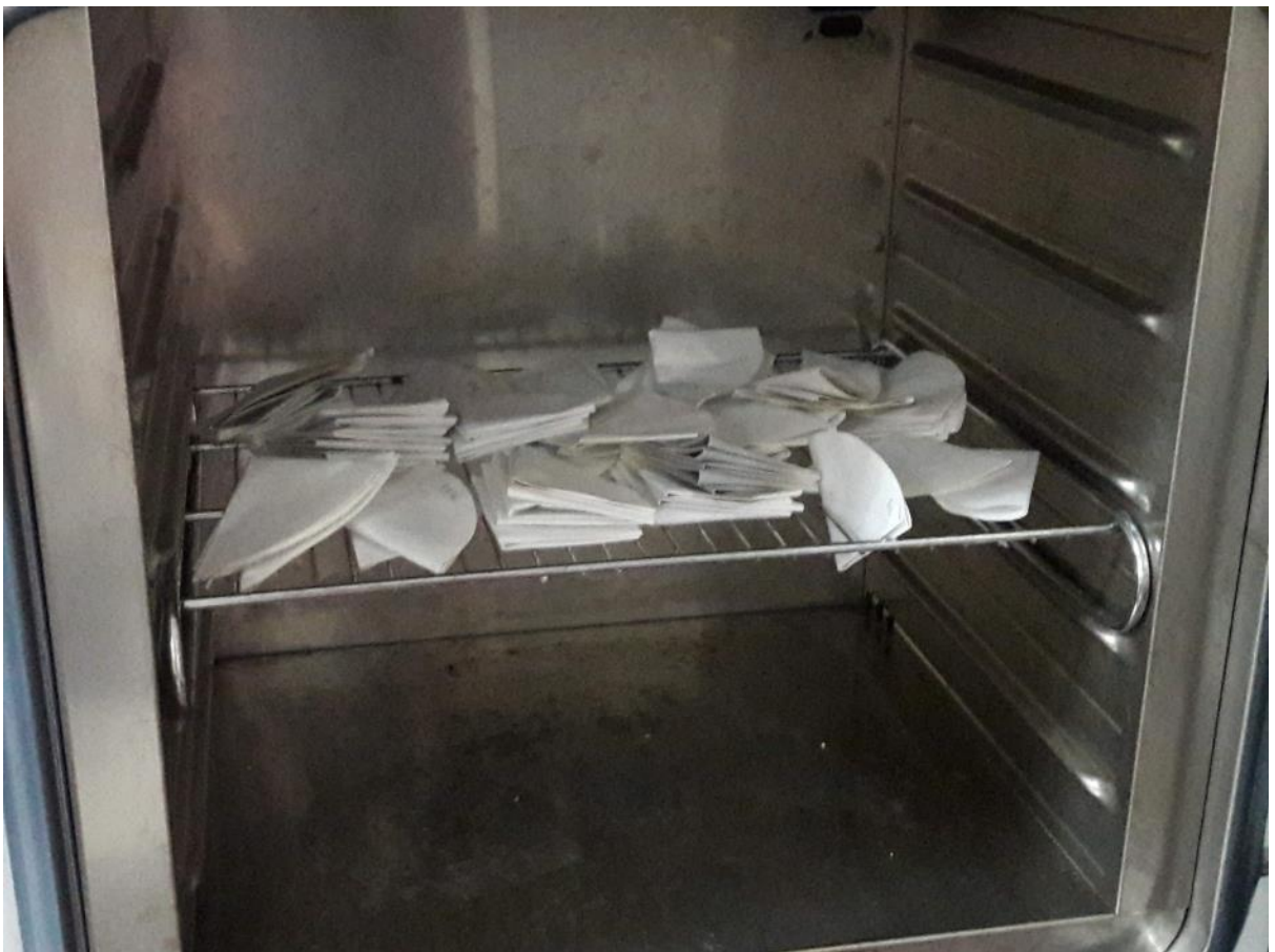
Image 8: Filtered sediments ready to dry in oven at 104 degree Celsius
