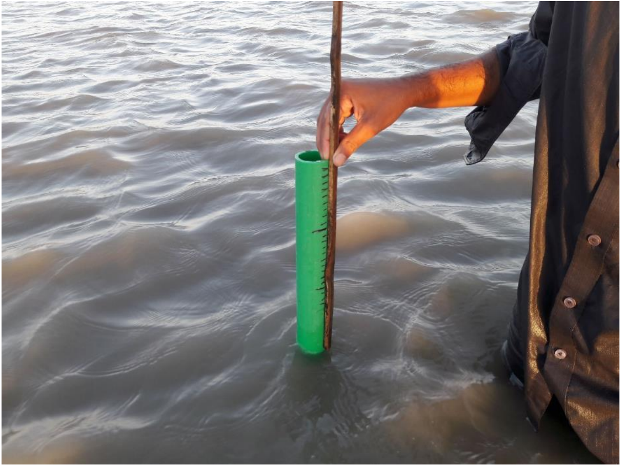
Image 3: Sediment deposition measurement inside the beel.
