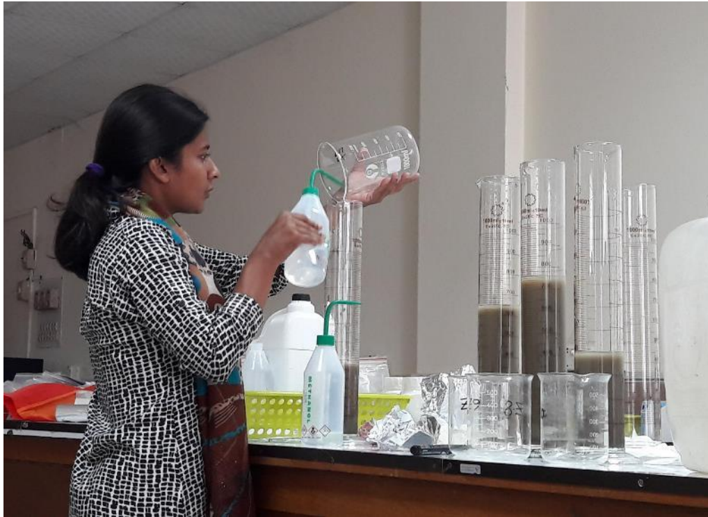
Image 6: Hydrometer tests to determine soil texture
