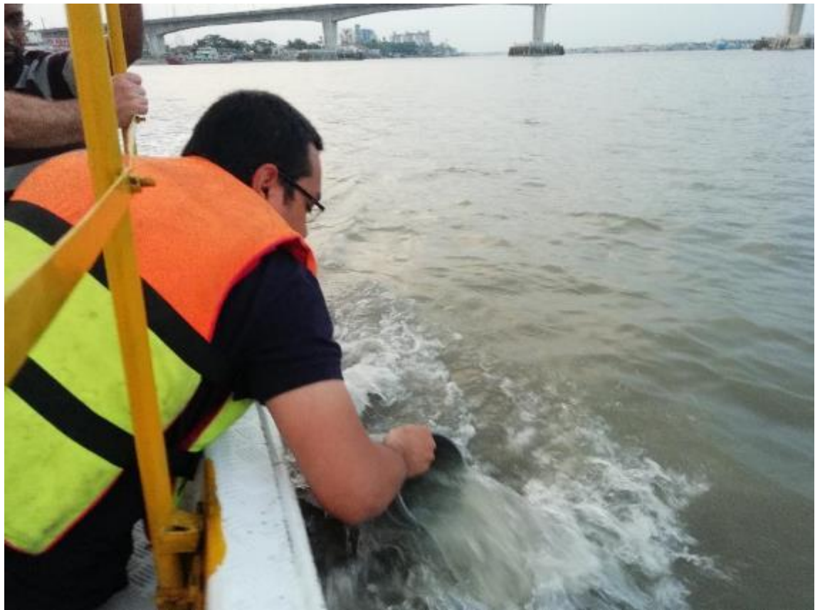
Image 40: Water sample collection at Rupsa River with settling tube
