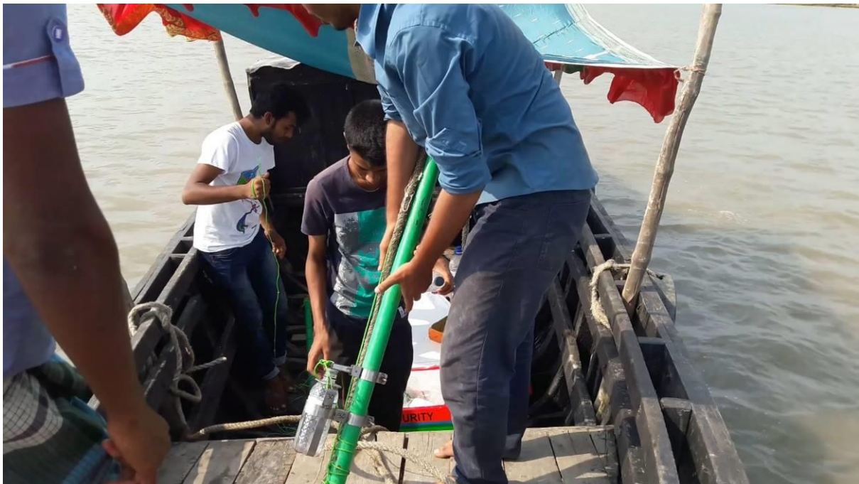
Figure 6: Sediment sample collection by Sediment sampler
