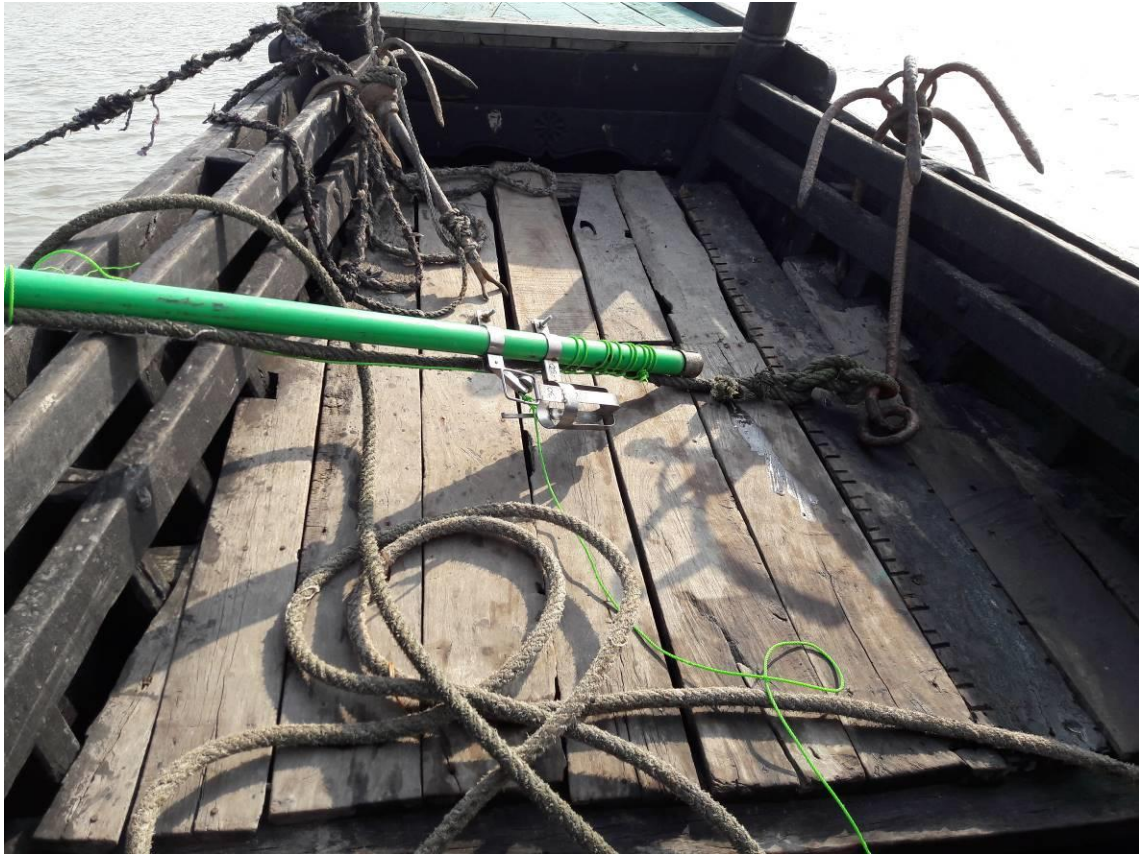
Figure 5: Sediment sampler and it's sampling arrangement
