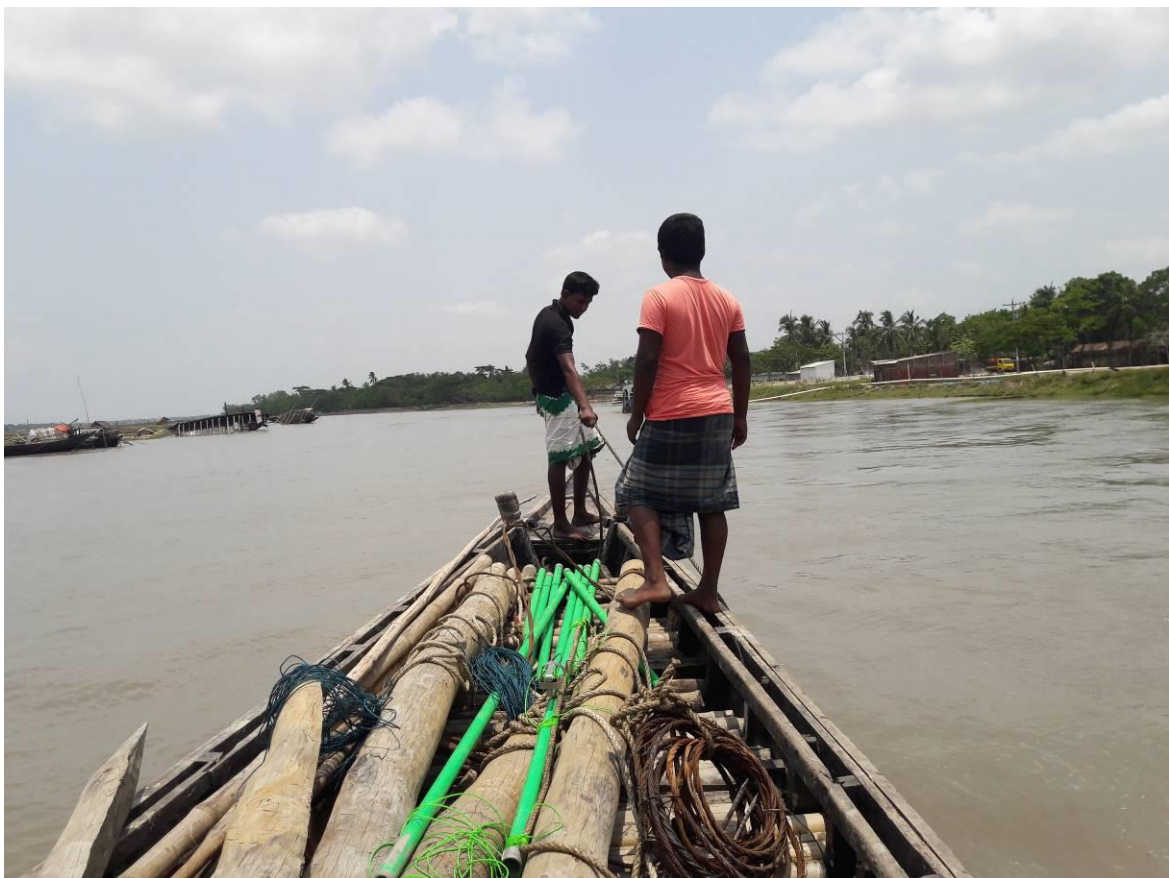
Figure 4: Depth measurement by anchoring rope
