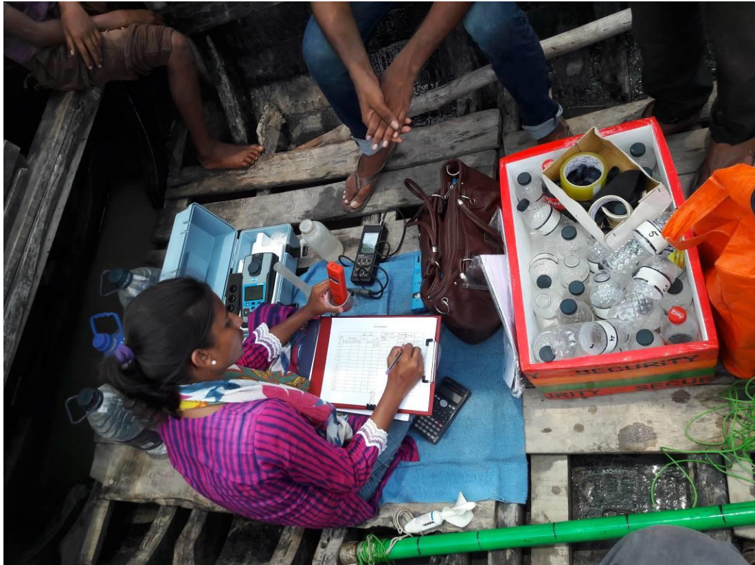
Figure 9: Data entry from various meters (EC meter, pH meter, Multi meter etc.)
