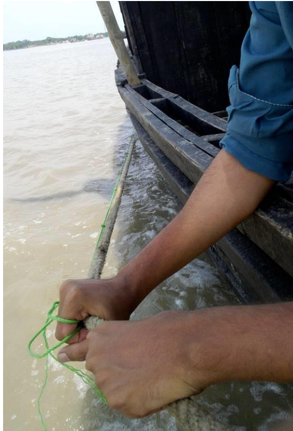
Figure 7: The inclination of the sampling rope during measurement due to high velocity
